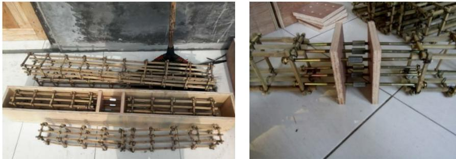
Figure 1. Bamboo reinforcements.
