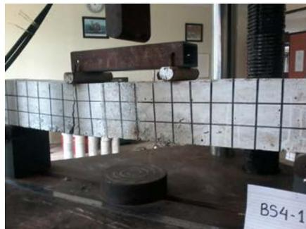
**Figure 6.** Crack pattern in BS4 beam.
