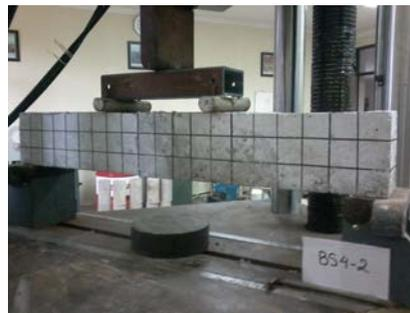
Figure 2. Four-point bending test.
