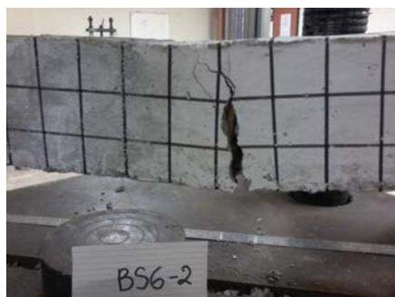
**Figure 7.** Crack pattern in BS6 beam
