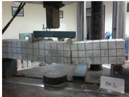
**Figure 5.** Crack pattern in BK beam.
